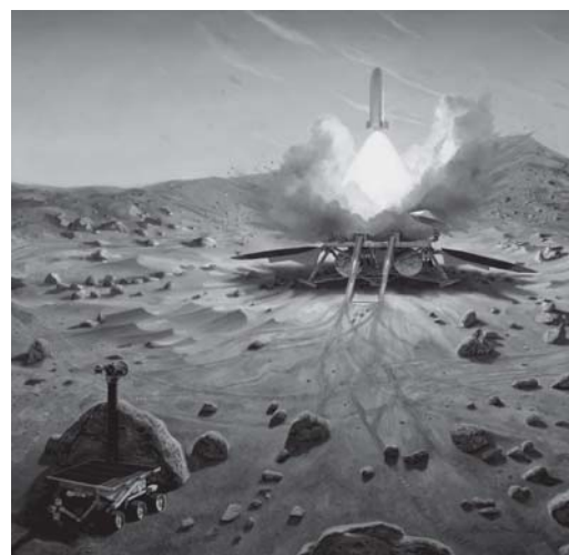
Figure 3. Artist's conception of Mars Sample Return (MSR) mission, where samples collected by rovers will be launched into Mars orbit, to be captured by an Earth-launched return vehicle. The priority for MSR has been moved up by the current NASA Science Director, but MSR still seems likely to be later than 2020.
